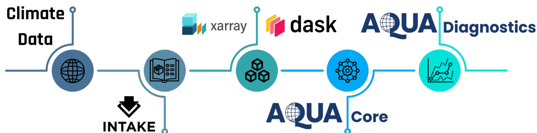
Figure 1. A scheme of the AQUA core dependencies and the separation between the AQUA core and the diagnostics. Climate data are the input for the AQUA code. Intake is then used to create data catalogs. AQUA leverages Xarray and Dask to enable lazy access computation. The AQUA framework is the part devoted to data access and process. Finally AQUA Diagnostics, a diagnostic suite based on the AQUA framework, is introduced (Paper II)
