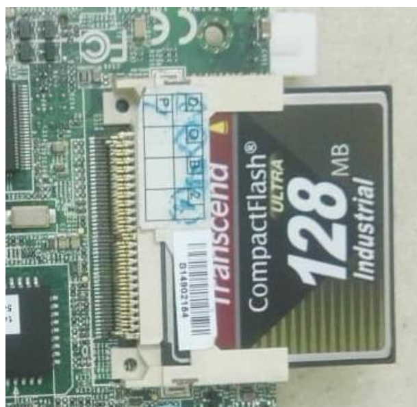
121 122 Figure A1: Close-up view of the PFM-540I PC/104-plus platform interface showcasing the industrial-grade Transcend 123 128 MB CompactFlash (CF) card used for system boot and data storage.
