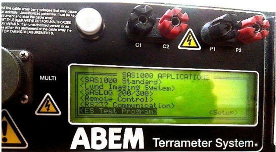
Figure 6: The Resistivity meter with functioning LCD display after the restoration
