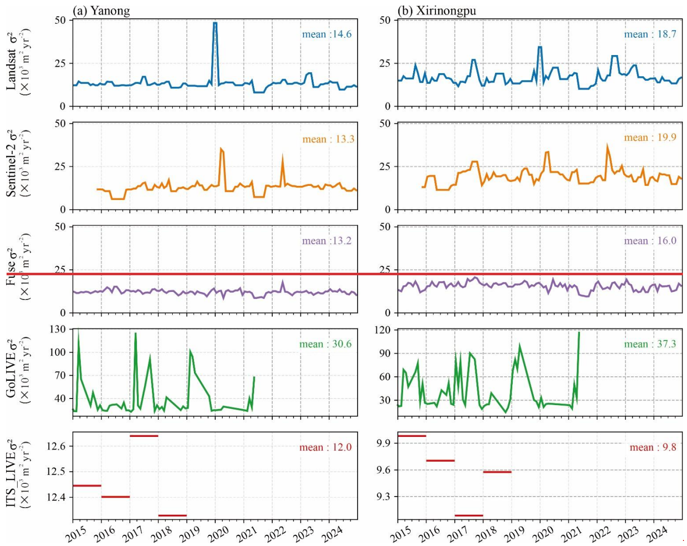
Figure 5: (a) Yanong Glacier; (b) Xirinongpu Glacier — variance of the Landsat velocity results, Sentinel-2 velocity results, fused results, GoLIVE dataset, and ITS_LIVE dataset.
