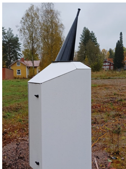
Figure 2. A termination hood (Vaisala CL61TERMHOOD) placed on top of the CL61 in Hyytiälä
