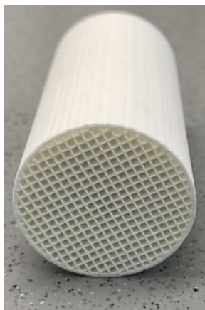
Figure S1 Photograph of the ceramic honeycomb body ( \text{\O} 25,4 \times 50\text{mm} ) used as substrate for Na 2 SO 3 coating in this study.
