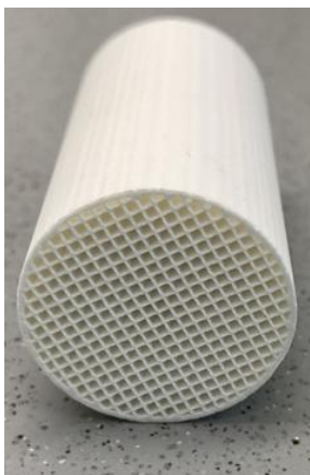
Figure S1 Photograph of the ceramic honeycomb body ( \text{\O} 25,4 \times 50\text{mm} ) used as substrate for \text{Na}_2\text{SO}_3 coating in this study.
