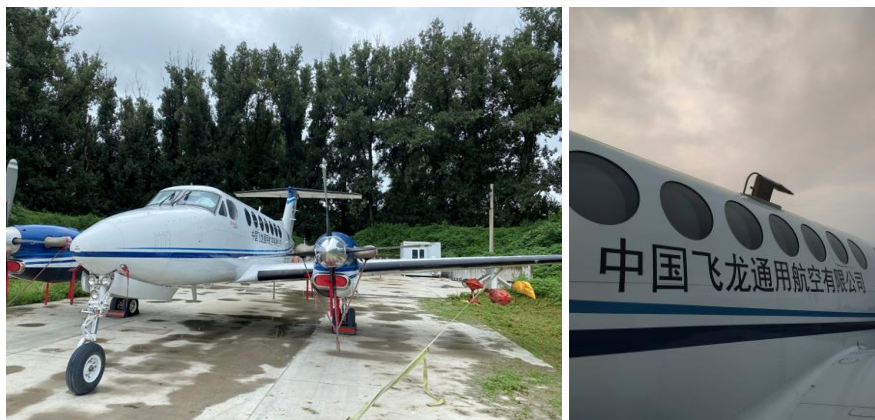
150 Figure 3: Photograph of the airplane (left) and the sampling inlet on the airplane (right)
