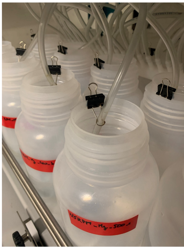
Figure A 1: Photograph of the setup with tubing maintained to each bottle rim with a binder clip. The air splitter apparatus can be distinguished in the background.
