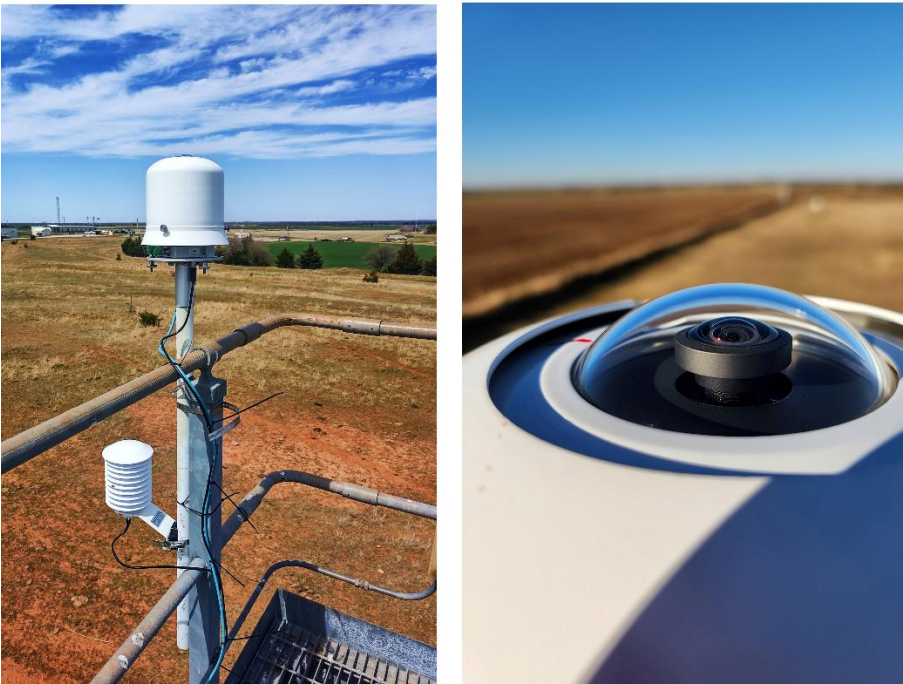
65 Figure 1: (Left) The ARM All-Sky-Imager (ASI) mounted at the Southern Great Plains (SGP) central site and (right) zoom on the ASI housing and fish-eye lens.
