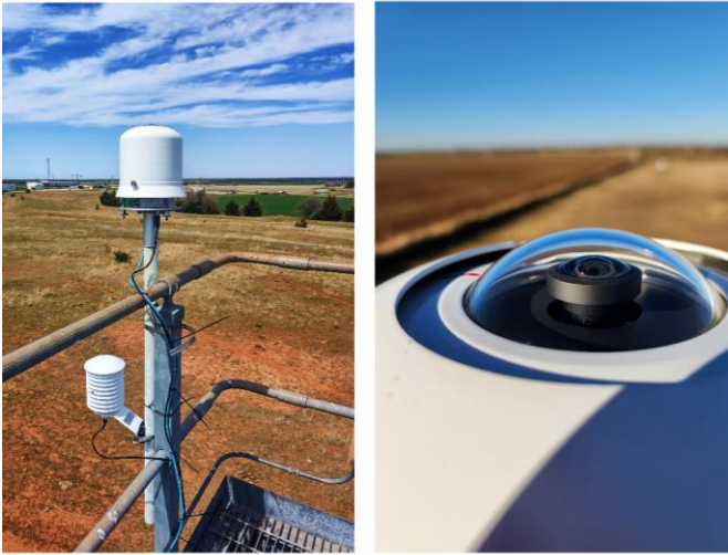
Figure 1: (Left) The ARM All-Sky-Imager (ASI) mounted at the Southern Great Plains (SGP) central site and (right) zoom on the ASI housing and fish-eye lens.
