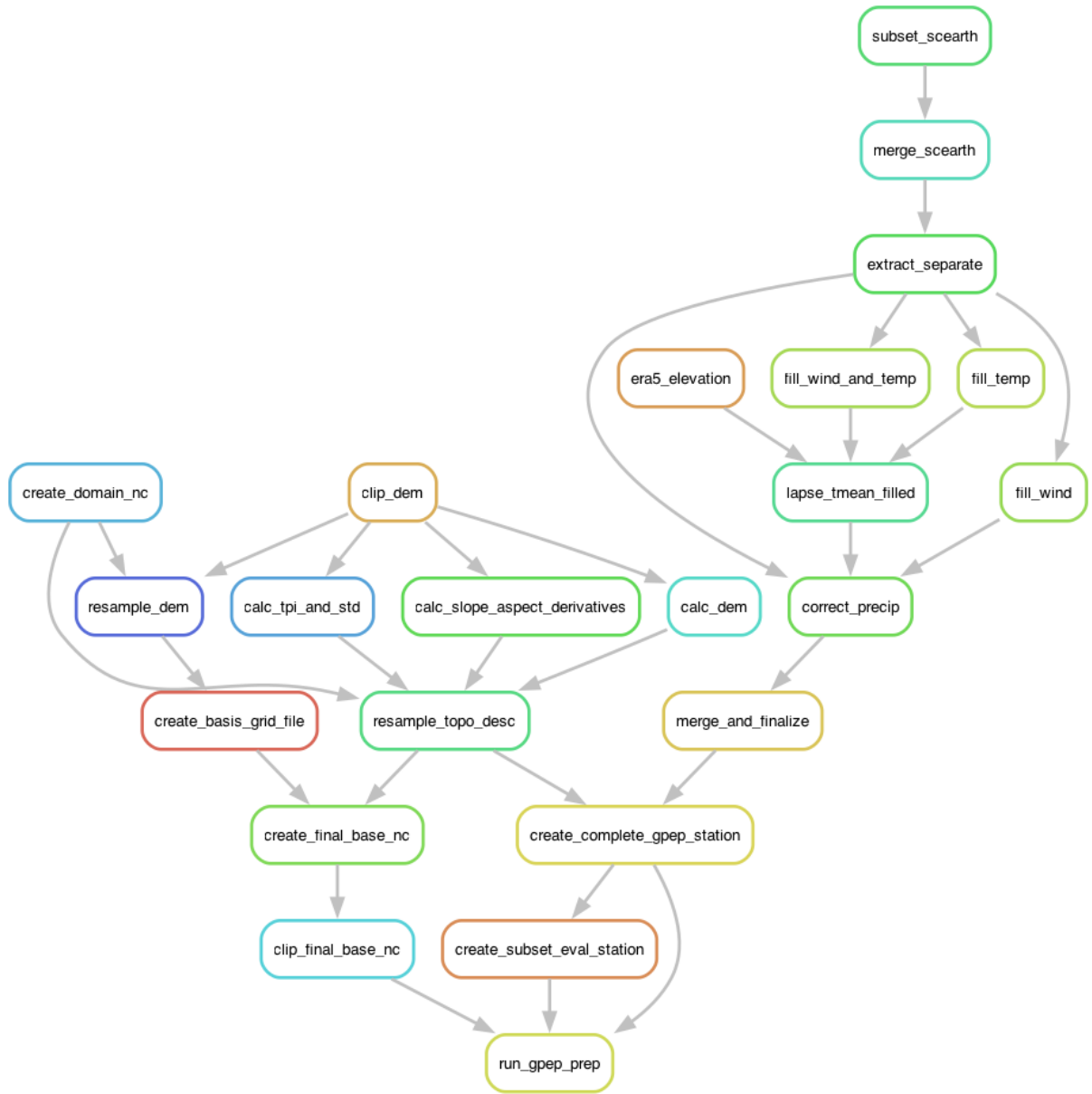
Figure 1: Autogenerated Snakemake workflow image example depicting static input data generation for GPEP. The workflow orchestrates a series of preprocessing steps to prepare gridded and meteorological station input data.
