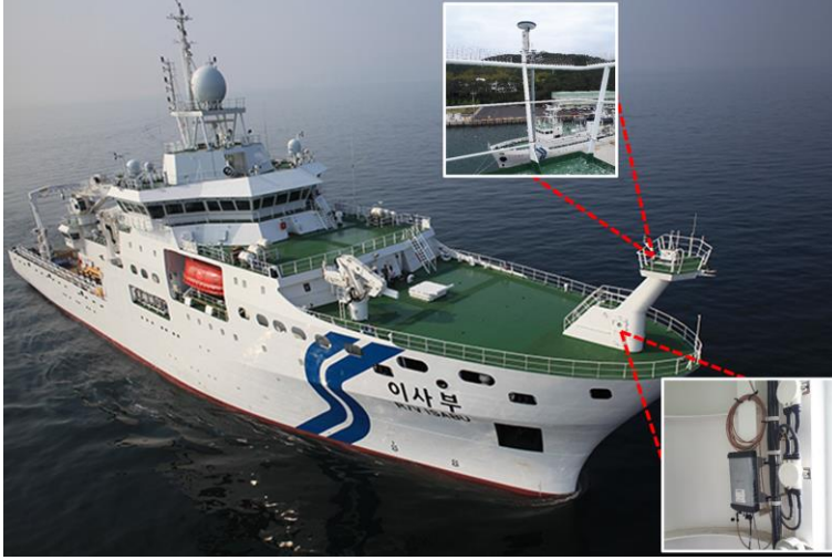
Figure 1. The global navigation satellite system (GNSS) antenna and receiver are installed on the foremast of the research vessel ISABU.
