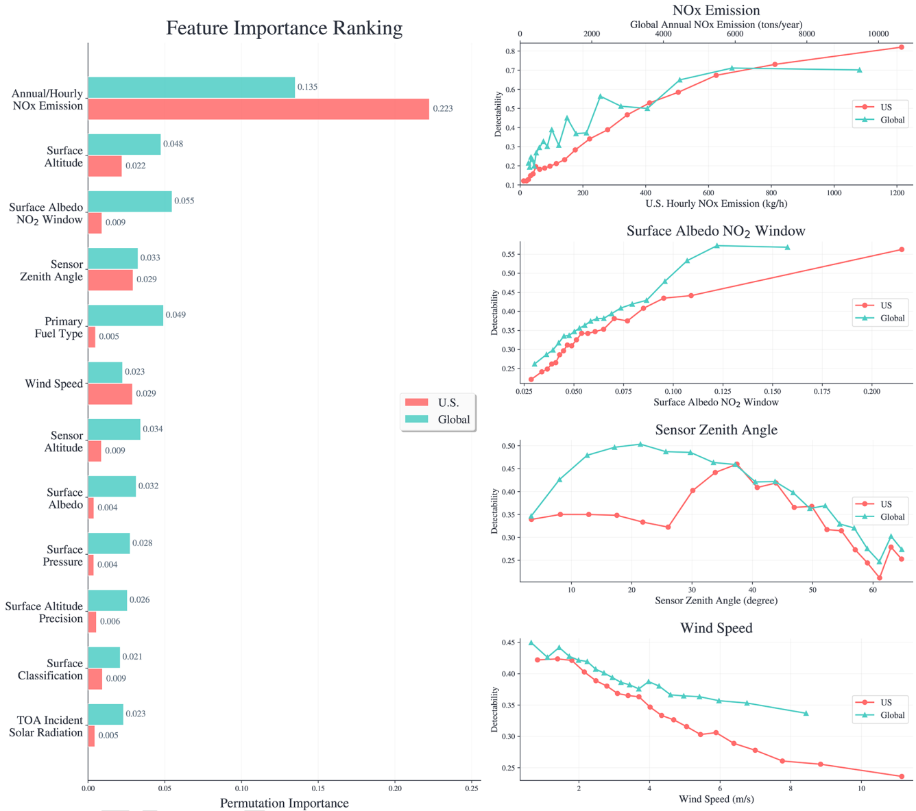
Figure 10. Feature importance and detectability analysis for TROPOMI-based NO 2 models at US (red) and global (teal) scales. Left: ranked permutation importance for the top 12 features, sorted by the sum of US and global importance and computed on the held-out test split of the dataset. Right: detectability as a function of NO x emission rate, surface albedo (NO 2 window), sensor zenith angle, and wind speed, computed on the dataset. Binning uses a quantile-based strategy (1st–99th percentile) to ensure balanced feature distribution and avoid extreme values. Dataset: modeling subset (Sect. 3.3; 171 US plants, n = 189\,713 observations; 1065 global plants, n = 161\,118 observations); the held-out test split contains n = 37\,943 US and n = 32\,224 global observations.
