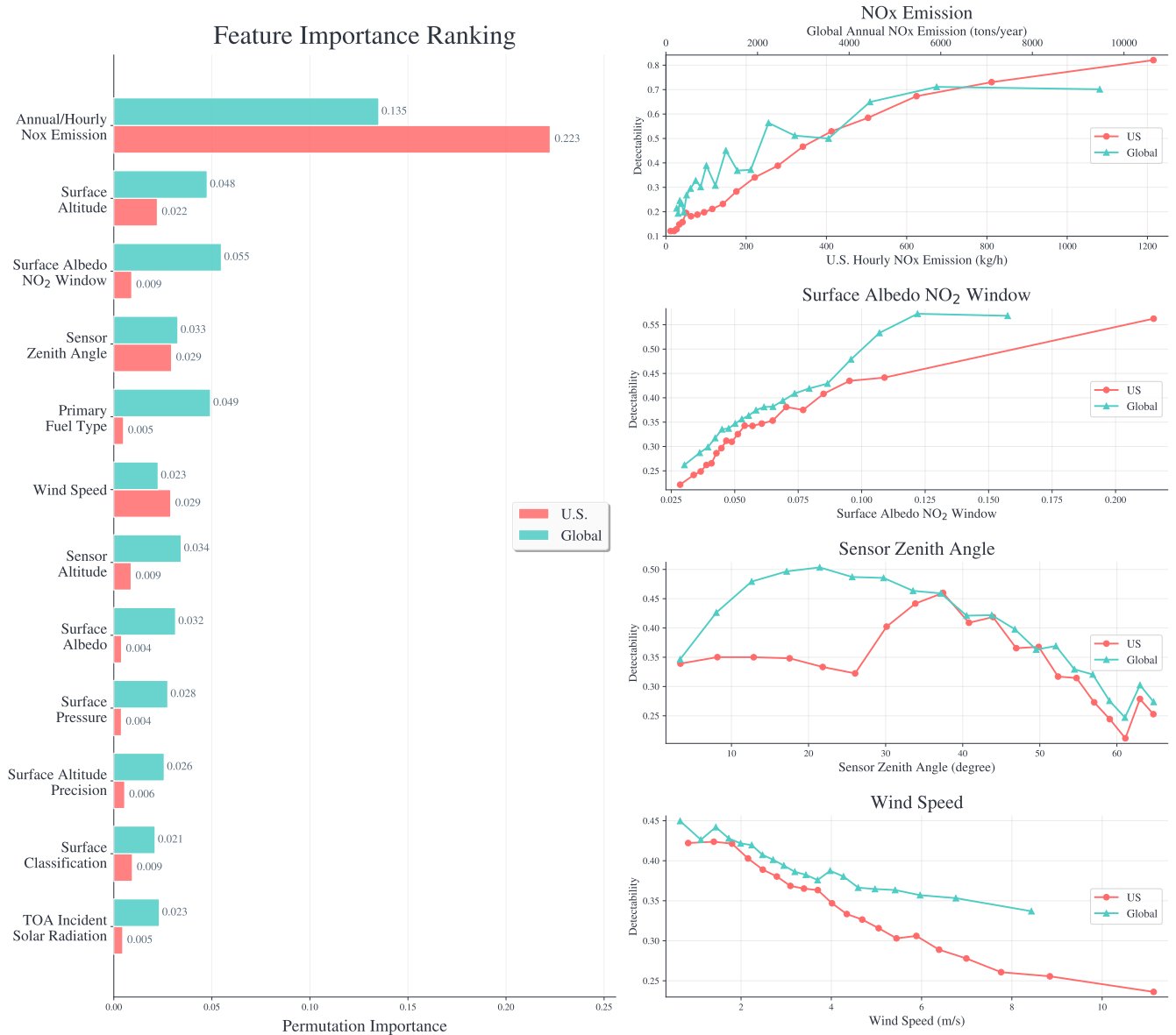
Figure 9. Feature importance and detectability analysis for TROPOMI-based NO 2 models at U.S. (red) and global (teal) scales. Left: ranked permutation importance for the top 12 features, sorted by the sum of U.S. and global importance and computed on the held-out test split of the dataset. Right: detectability as a function of NO x emission rate, surface albedo (NO 2 window), sensor zenith angle, and wind speed, computed on the dataset. Binning uses a quantile-based strategy (1st–99th percentile) to ensure balanced feature distribution and avoid extreme values. Dataset: modeling subset (Sect. 3.3; 171 U.S. plants, n = 189,713 observations; 1,065 global plants, n = 161,118 observations); the held-out test split contains n = 37,943 U.S. and n = 32,224 global observations.
