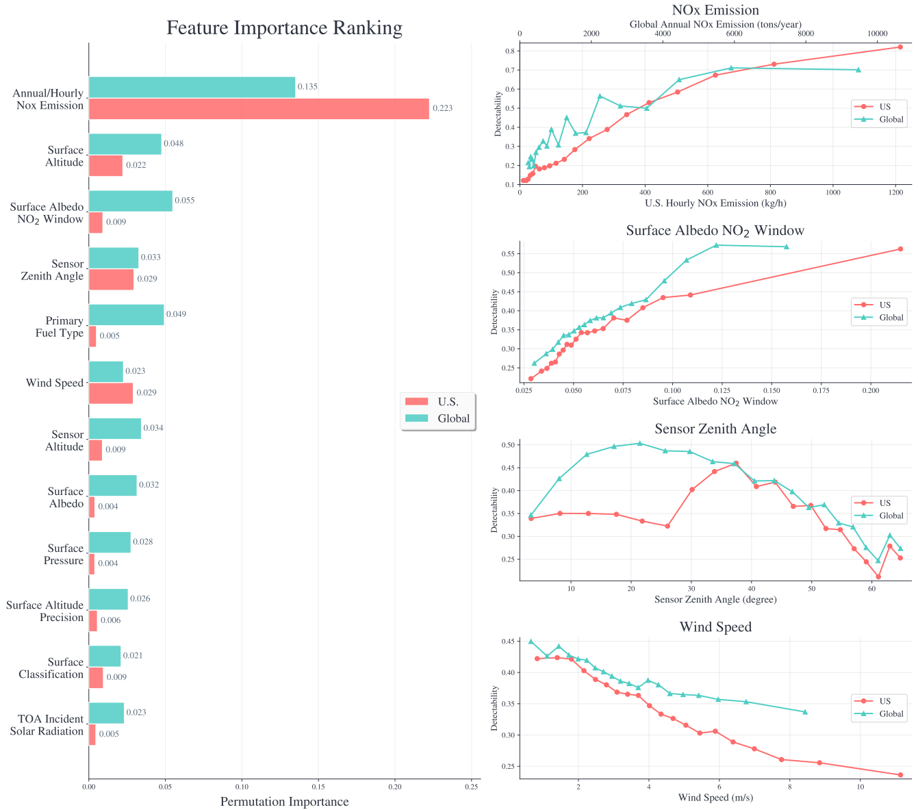
Figure 10. Feature importance and detectability analysis for TROPOMI-based NO 2 models at U.S. (red) and global (teal) scales. Left: ranked permutation importance for the top 12 features, sorted by the sum of U.S. and global importance and computed on the held-out test split of the dataset. Right: detectability as a function of NO x emission rate, surface albedo (NO 2 window), sensor zenith angle, and wind speed, computed on the dataset. Binning uses a quantile-based strategy (1st–99th percentile) to ensure balanced feature distribution and avoid extreme values. Dataset: modeling subset (Sect. 3.3; 171 U.S. plants, n = 189,713 observations; 1,065 global plants, n = 161,118 observations); the held-out test split contains n = 37,943 U.S. and n = 32,224 global observations.
