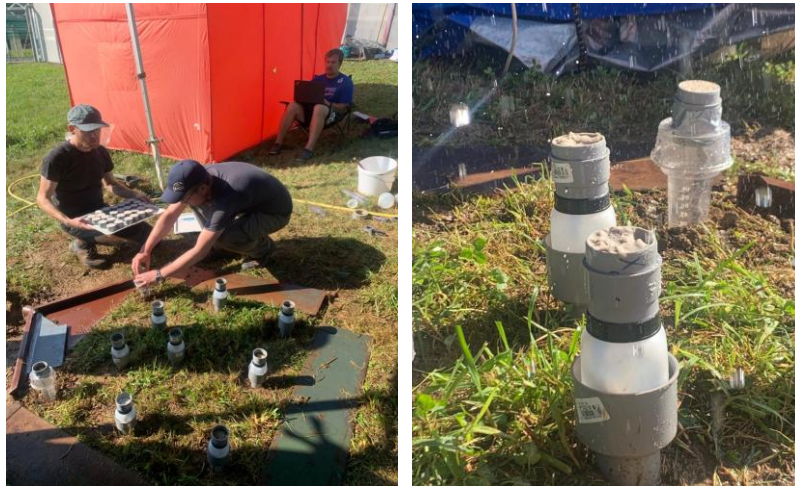
Figure 5: Splash cups installation prior to the experiment (left) and during the simulation (right)
