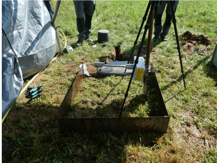
Figure 4: Thies disdrometer measurement with the Prague Portable Rainfall Simulator
