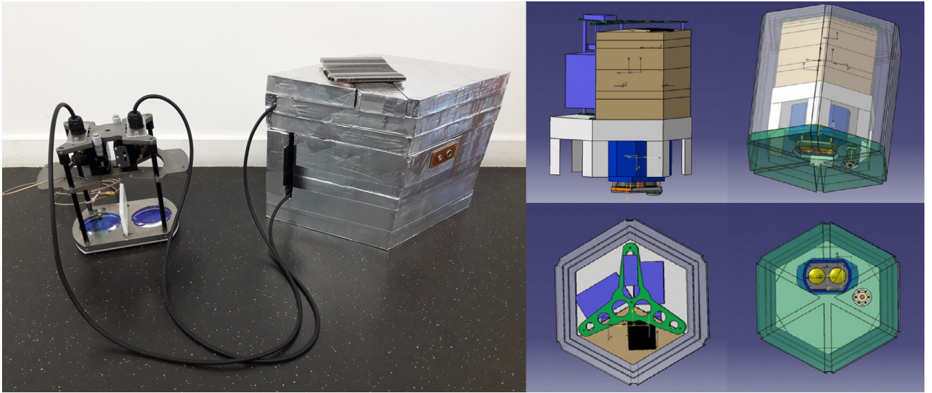
Figure 2. Picture (left) and 3D drawing (right) of BeCOOL microlidar. The optical head (OH) equipped with two lenses can be seen in the lower (“cold”) part of the gondola. The two other boxes with diamond shape are shown in brown in the upper (“hot”) part of the gondola, sharing the volume with the Zephyr electronic, other instruments and the batteries.
