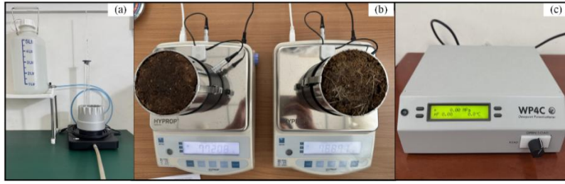
Fig. 2. Laboratory measurement instruments. (a) KSAT Hydraulic conductivity measurement; (b) HYPROP 2 Evaporation experiment; (c) WP4C Dew point water potential meter.
