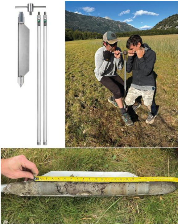
195 Figure 3. Russian Peat Auger (RPA) used in the field. The auger is pushed into substrate (top-right), and rotated to close the gate, isolating the sediment core from the substrate.
