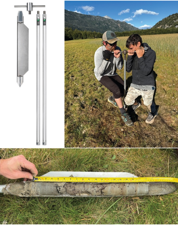
Figure 4. Russian Peat Auger (RPA) used in the field. The auger is pushed into substrate (top-right), and rotated to close the gate, isolating the sediment core from the substrate.
