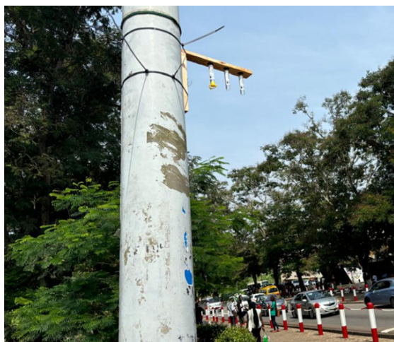
245 Figure 4: Deployed Palmes diffusion tubes mounted on site: one blank sample and two tubes measuring in duplo.
