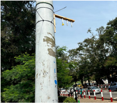
Figure 4: Deployed Palmes diffusion tubes mounted on site: one blank sample and two tubes measuring in duplo.
