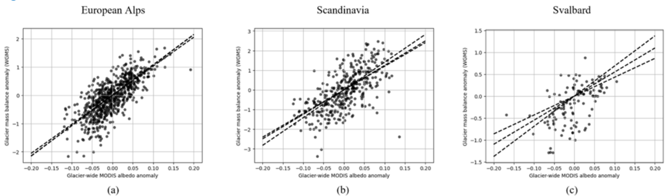
Figure 5: Glacier-wide summer albedo annual anomalies versus annual glacier mass-balance anomalies from WGMS observations for glaciers in the European Alps (a), Scandinavia (b), and Svalbard (c). Dashed lines show the linear relationships obtained from the 3-fold cross-validation, where the mass-balance–albedo anomaly gradients ( \frac{db}{d\alpha} ) are estimated iteratively using two-thirds of the glaciers in each region. The spread between dashed lines reflects the variability of the gradient across the three cross-validation folds.
