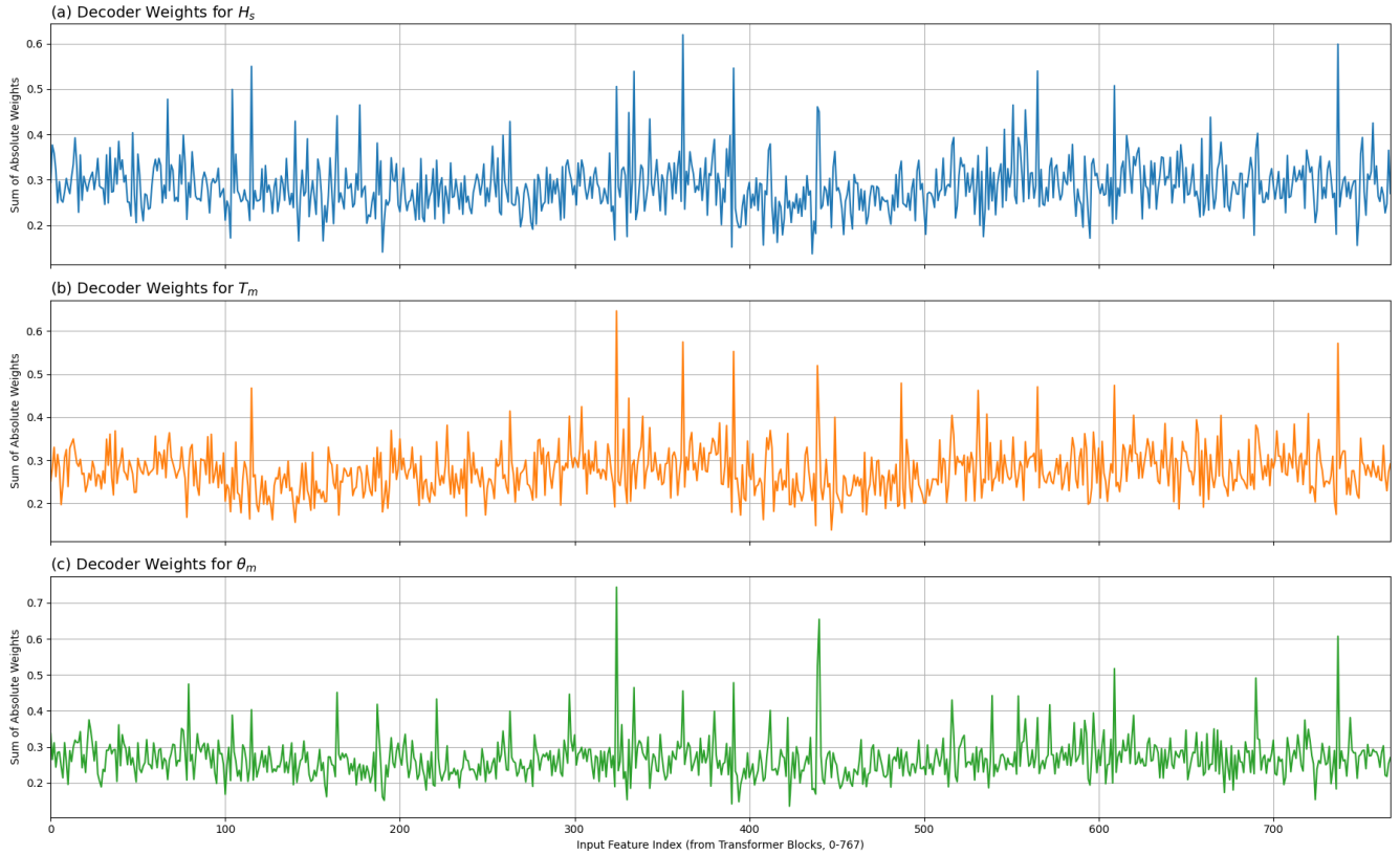
Figure 3. Decoder weight magnitude for individual latent features. The sum of absolute decoder weights connecting each of the 768 latent features (x-axis) to the three physical output variables: (a) H_s , (b) T_m , and (c) \theta_m .
