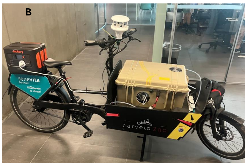
Figure 1: (a) Model Rendering of the Portable-TOF-CIMS, (b) Portable-TOF-CIMS in standalone operation on a battery pack ready for deployment with cargo e-Bike.
