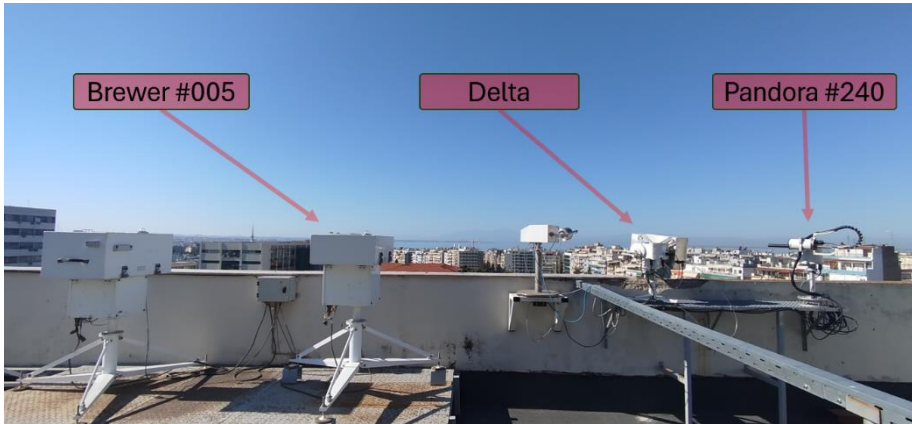
135 Figure 1: The measurement site of LAP.AUTH and the three collocated ground-based instruments used in this study: Brewer spectrophotometer #005 (left), Delta UV-VIS DOAS system (centre), and Pandora #240 (right).
