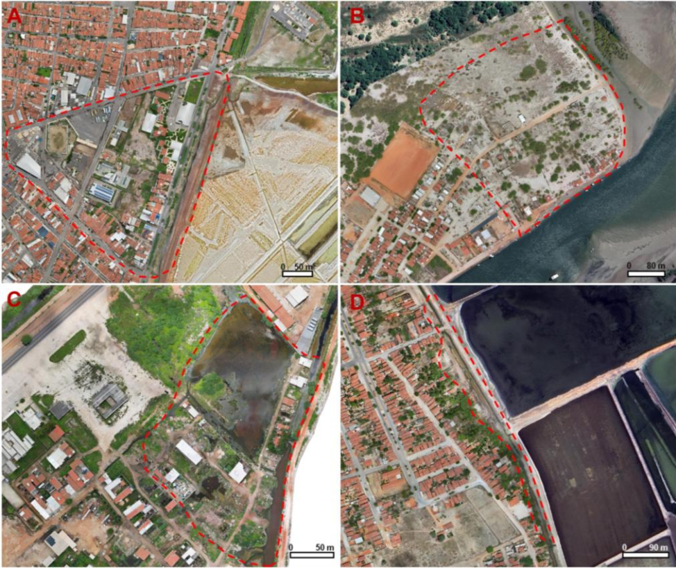
Figure 10: Photographic records of the main areas indicated by the model as extremely high risk. It is noteworthy to observe the lowering of the mapped areas, especially Areia Branca, where flooding was verified in the field. A - section of the urban area of Macau with the most susceptible area; B - section of the urban area of Porto do Mangue with a low-lying portion prone to flooding; C - urban area of Areia Branca with flooding boundaries; and D - urban area of Grossos with channels prone to overflowing. Photographs by the authors (2025).
