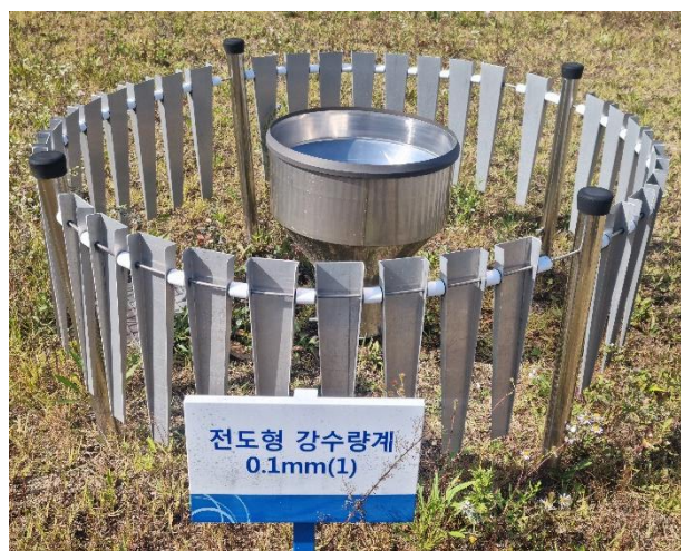
172 Figure 3: (a) Tipping-bucket rain gauge (0.1 mm) and (b) Weighing rain gauge (0.1 mm).
