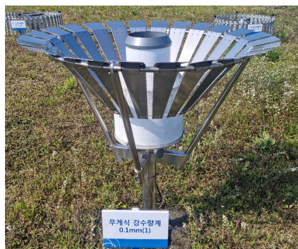
172 Figure 3: (a) Tipping-bucket rain gauge (0.1 mm) and (b) Weighing rain gauge (0.1 mm).
