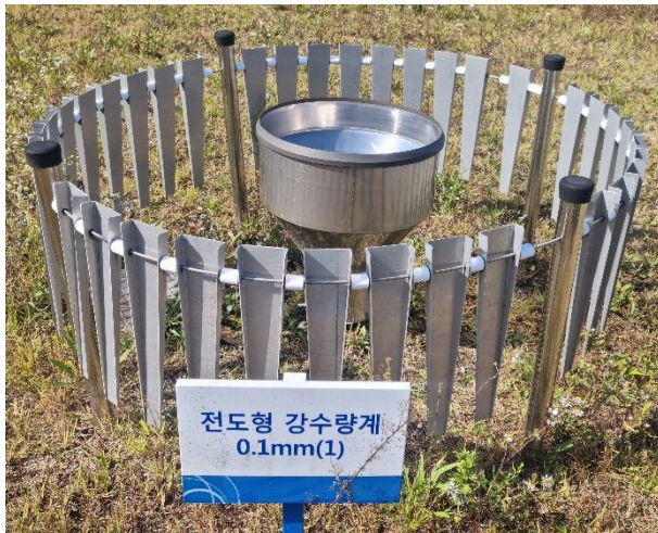
176 Figure 3: (a) Tipping-bucket rain gauge (0.1 mm) and (b) Weighing rain gauge (0.1 mm).
