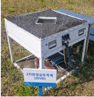
169 Figure 2: Two-dimensional video disdrometer.
