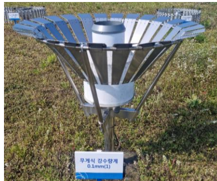
175 Figure 3: (a) Tipping-bucket rain gauge (0.1 mm) and (b) Weighing rain gauge (0.1 mm).
