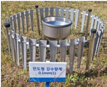
175 Figure 3: (a) Tipping-bucket rain gauge (0.1 mm) and (b) Weighing rain gauge (0.1 mm).
