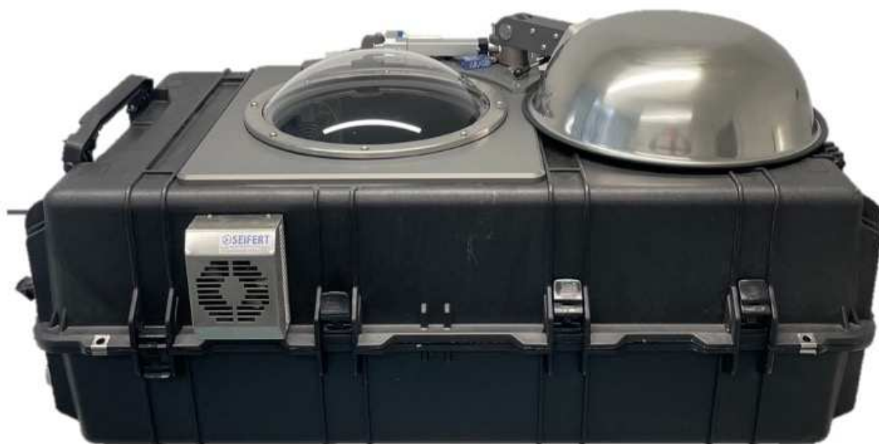
Figure A2. Photograph of a fully assembled EM27/SUN weatherproof enclosure.
