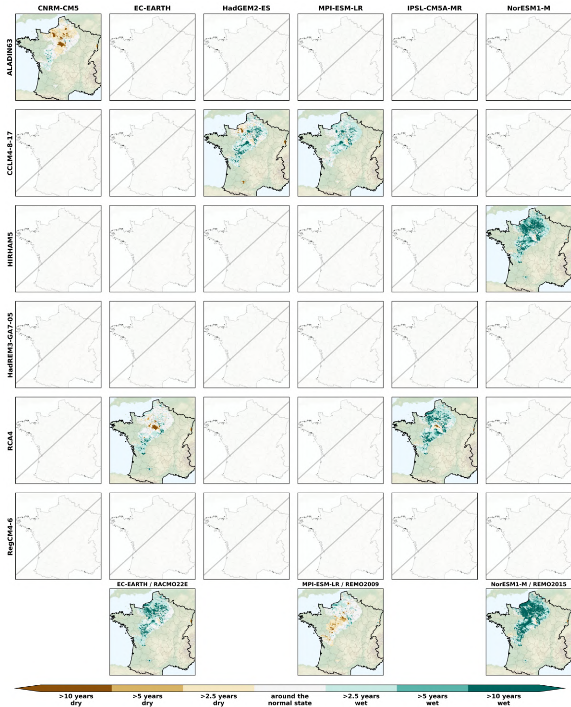
Figure B6. Spatial distribution of the SPLI median over the AquifR domain under the RCP4.5 on the long-term horizon (2071-2099) , following the different GCM (in column) / RCM (in line) combination. The last line corresponds to couples where RCMs are used only once.
