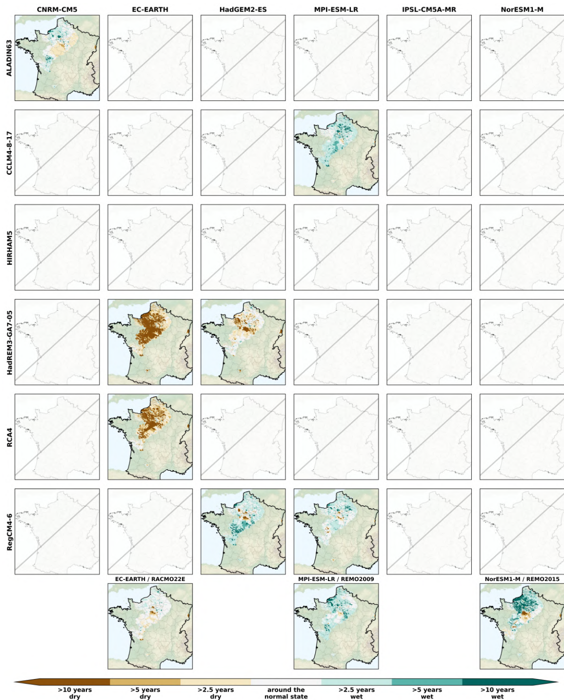
Figure B2. Spatial distribution of the SPLI median over the AquifR domain under the RCP2.6 on the intermediate-term horizon (2041-2070) , following the different GCM (in column) / RCM (in line) combination. The last line corresponds to couples where RCMs are used only once.
