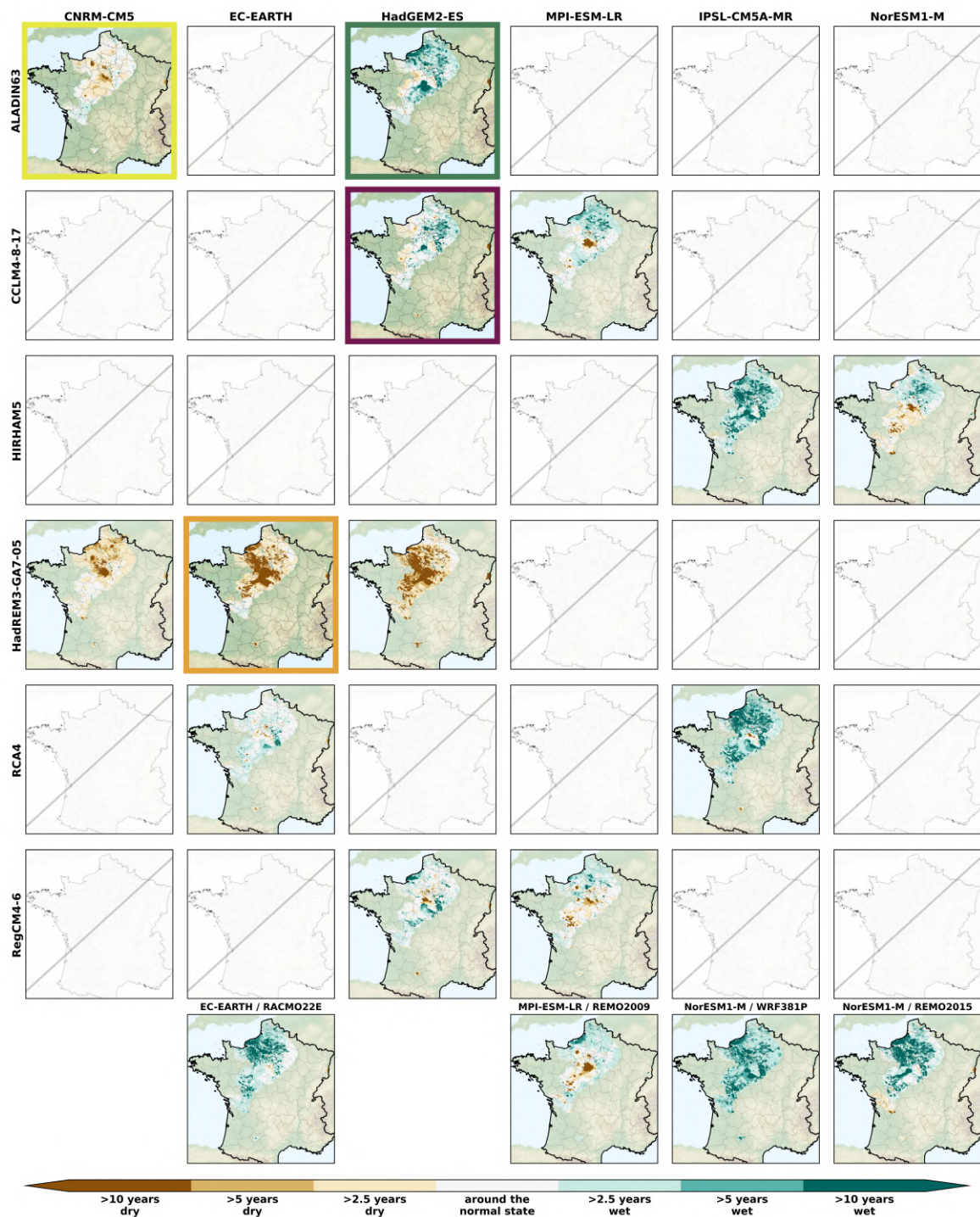
Figure B8. Spatial distribution of the SPLI median over the AquifR domain under the RCP8.5 on the intermediate-term horizon (2041-2070) , following the different GCM (in column) / RCM (in line) combination. The last line corresponds to couples where RCMs are used only once. The colored rectangles indicates the GCM/RCM couples corresponding to the storylines (see section 2.1).
