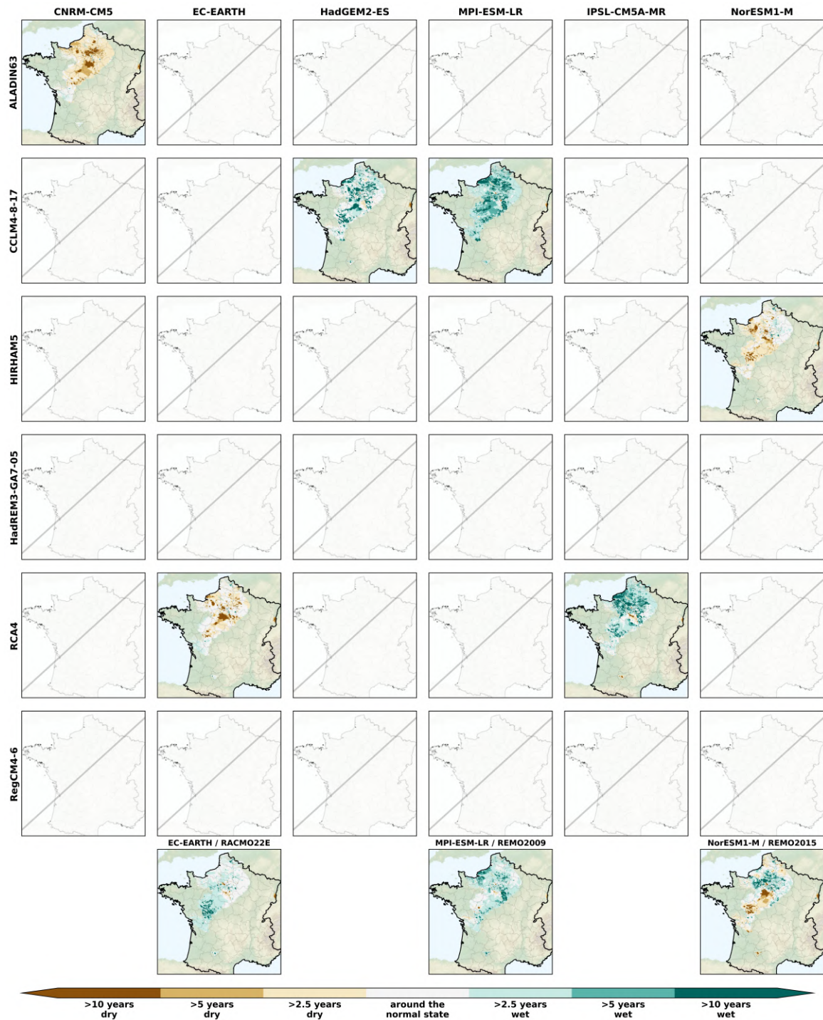
Figure B4. Spatial distribution of the SPLI median over the AquifR domain under the RCP4.5 on the short-term horizon (2021-2050) , following the different GCM (in column) / RCM (in line) combination. The last line corresponds to couples where RCMs are used only once.
