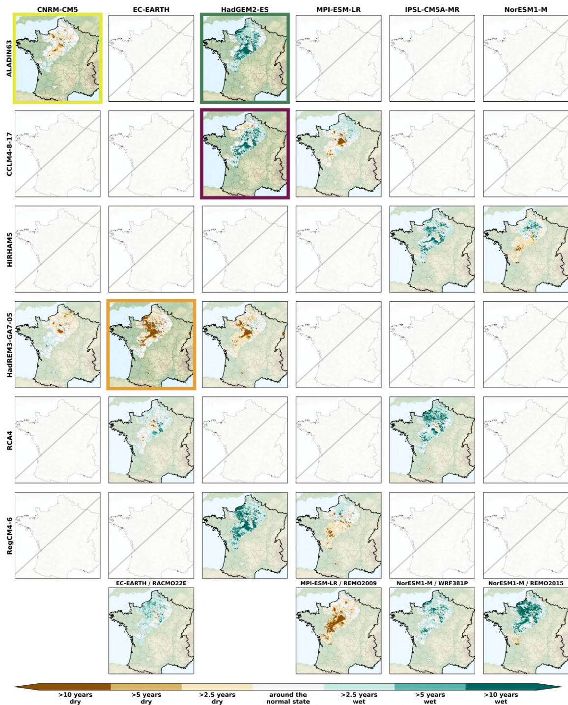
Figure B7. Spatial distribution of the SPLI median over the AquifR domain under the RCP8.5 on the short-term horizon (2021-2050) , following the different GCM (in column) / RCM (in line) combination. The last line corresponds to couples where RCMs are used only once. The colored rectangles indicates the GCM/RCM couples corresponding to the storylines (see section 2.1).
