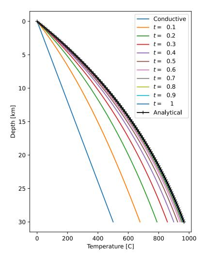
Figure 1: Comparison between numerical transient solution (colored lines) and analytical steady-state solution (black line with crosses).
