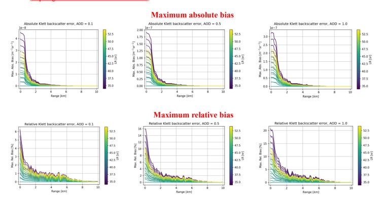
This analysis highlighted that the bias introduced in the backscatter retrievals by using a constant lidar ratio of 44 sr — even when the true lidar ratio varies between 34 and 54 sr — remains relatively small and does not significantly impact the shape or magnitude of the resulting backscatter profiles in most realistic scenarios. Therefore, recalculating the backscatter coefficient profiles for each lidar ratio is not
