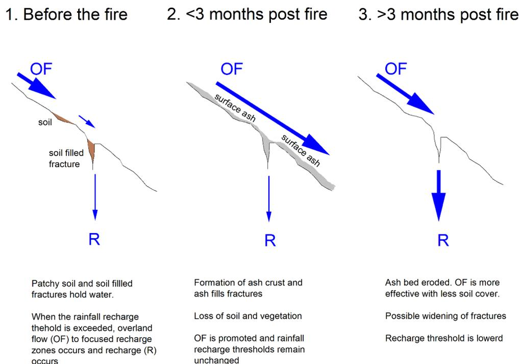
215 **Figure 8.** Conceptual figure of the recharge processes (1) before the fire (2) less than three months after the fire and (3) More than three months
