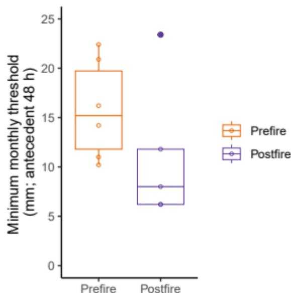
156 **Figure 6.** Minimum monthly rainfall recharge threshold (48 h, mm) for the pre fire (orange) and post fire (purple) periods
