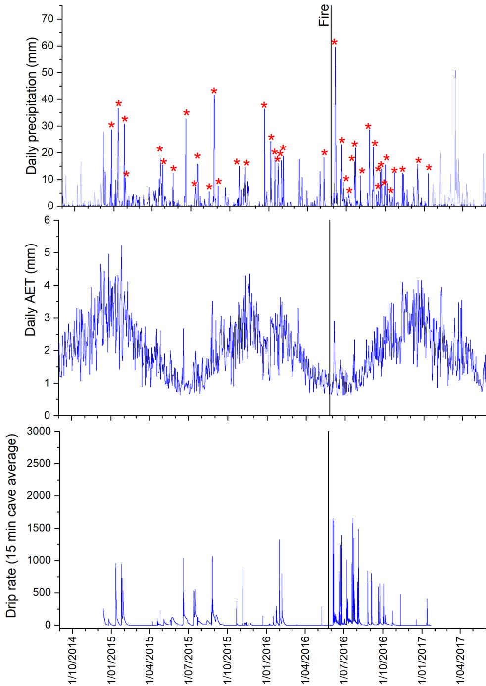
129 **Figure 3.** Daily precipitation (light blue when outside the monitoring period) with timing of recharge events shown by red asterisks, daily
