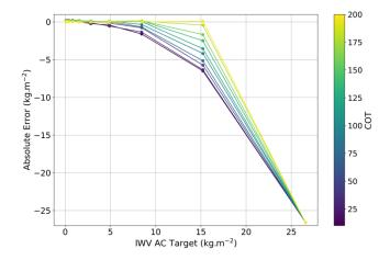
Caption (new file, page.13 Figure 5.): Same as figure 4 for the three spectral bands (1.04, 1.13 and 1.37  $\mu$ m) configuration but with a large uncertainty of 2000 m for the cloud base altitude identified as a non-retrieved parameter.
