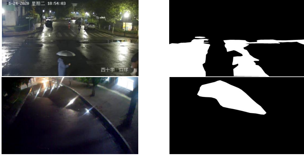
Figure 2: Samples and the flood area labels in the dataset, the white marked range is the flood extent. Data Samples–
