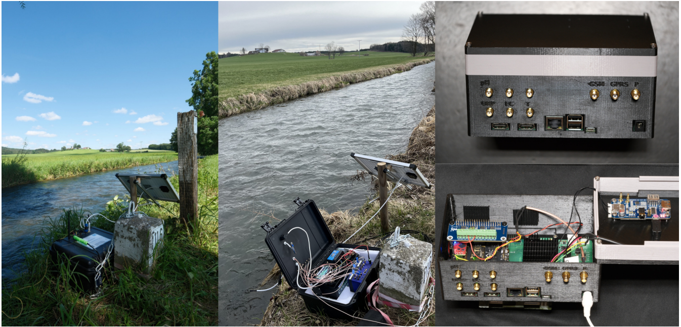
Figure 2. River water monitoring kit.
