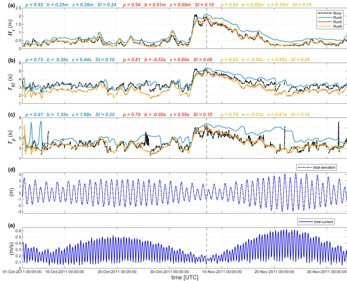
Figure A1: Comparison of the (a) significant wave height H_s , (b) mean period T_{0.2} and (c) peak period T_p between observations and the WW3 simulations (Run 4 without S_{uo} and tides, Run 5 with S_{uo} but without tides, Run 8 with S_{uo} and FES2014 tides) during October 2011 at Hay Point wave buoy (55032; water depth of 9 m), respectively. The error metrics are printed in blue, red
