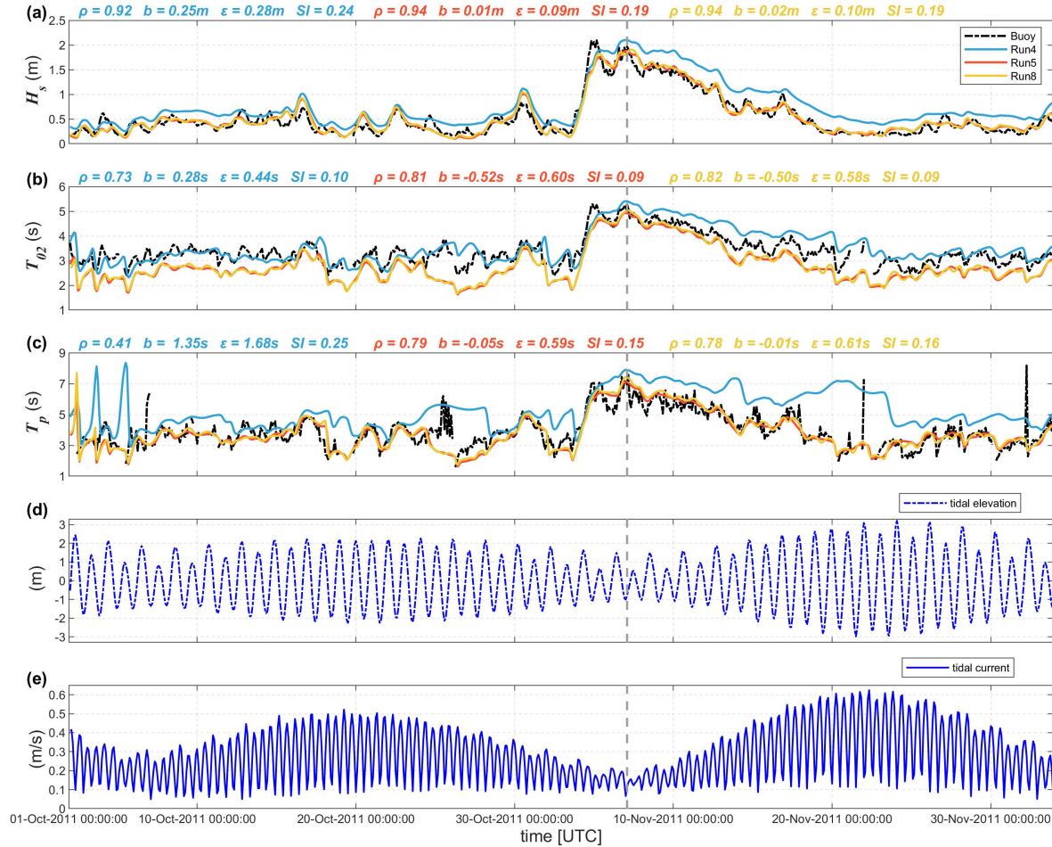
Figure A1: Comparison of the (a) significant wave height H_s , (b) mean period T_{0.2} and (c) peak period T_p between observations and the WW3 simulations (Run 4 without S_{uo} and tides, Run 5 with S_{uo} but without tides, Run 8 with S_{uo} and FES2014 tides) during October 2011 at Hay Point wave buoy (55032; water depth of 9 m), respectively. The error metrics are printed in blue, red and yellow colors, respectively. (d) and (e) represent the tidal elevation and tidal currents for October 2011 based on the FES2014 database, respectively. The vertical dashed line highlights the time instant analyzed in Fig. 12.
