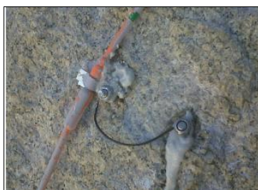
Figure 3: Photo of the jumper used to attached electrodes and take-out.
