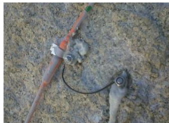
Photo 1: specially designed stainless-steel jumper used to attach the cable takeout onto the climbing bolt, with maximum electrical contact (duplicated electrode).
