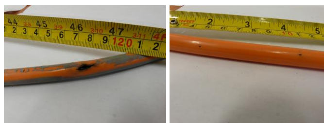
Photo 2: Effect of lightning on the ERT cables
