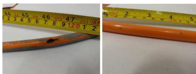
Photo 2: Effect of lightning on the ERT cables
