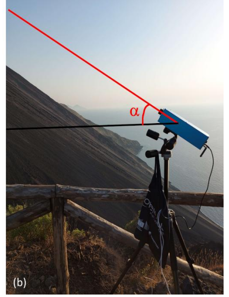
Figure 3: (a) Schematic geometrical configuration of VIRSO2 camera FOV. The camera is placed in C. (b) VIRSO2 camera at Stromboli (Italy). (Note that Earth curvature effects are ignored as generally the system operates on small scales ~10 km or so).
