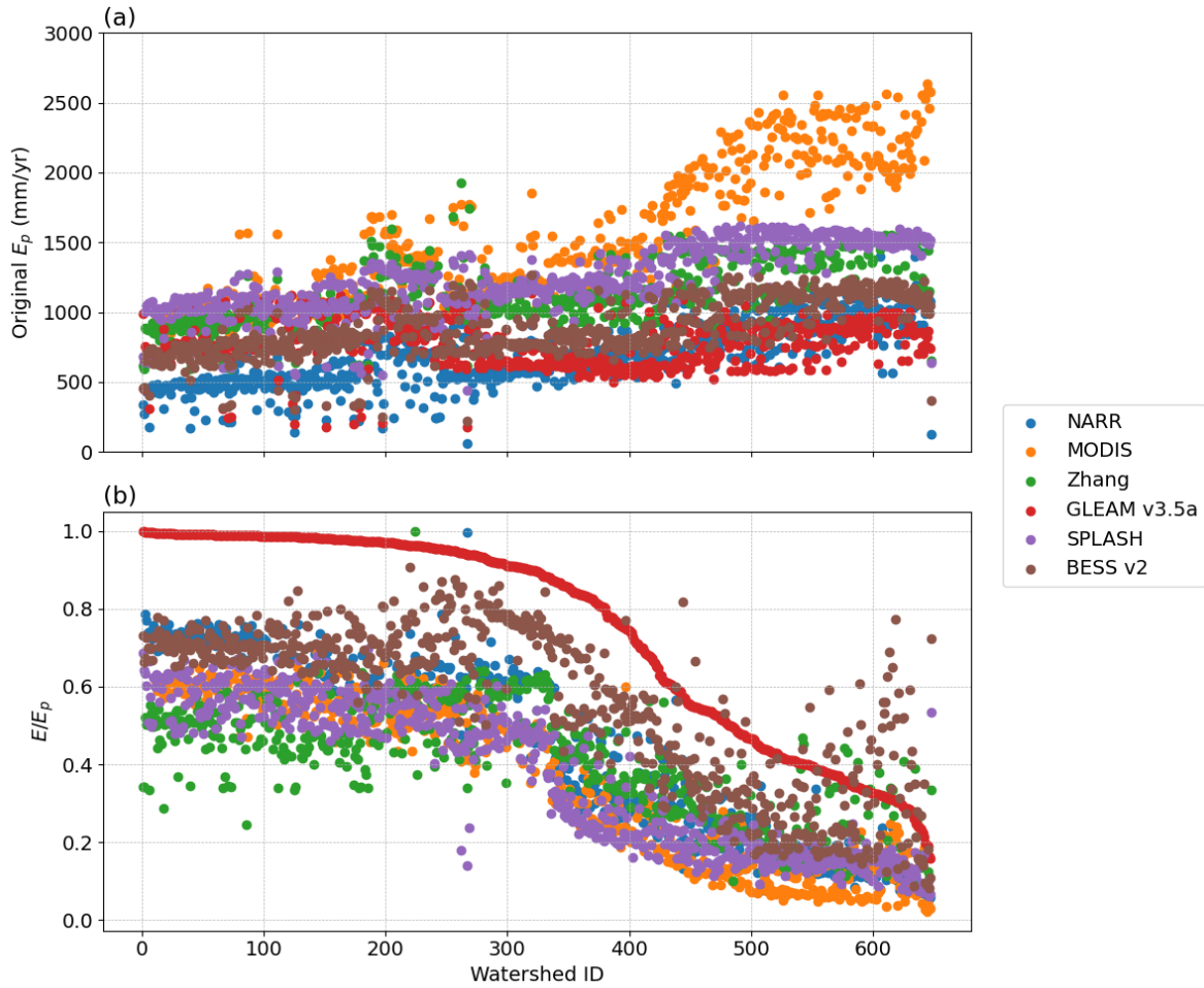
Figure 3: Original E_p for six data products: NARR, MODIS, Zhang, GLEAM v3.5a, SPLASH, and BESS v2 for 648 watersheds. (a) E_p values retrieved from the data products, and (b) E/E_p ratios retrieved from the data products. Watersheds are sorted in descending order according to GLEAM's E/E_p .
