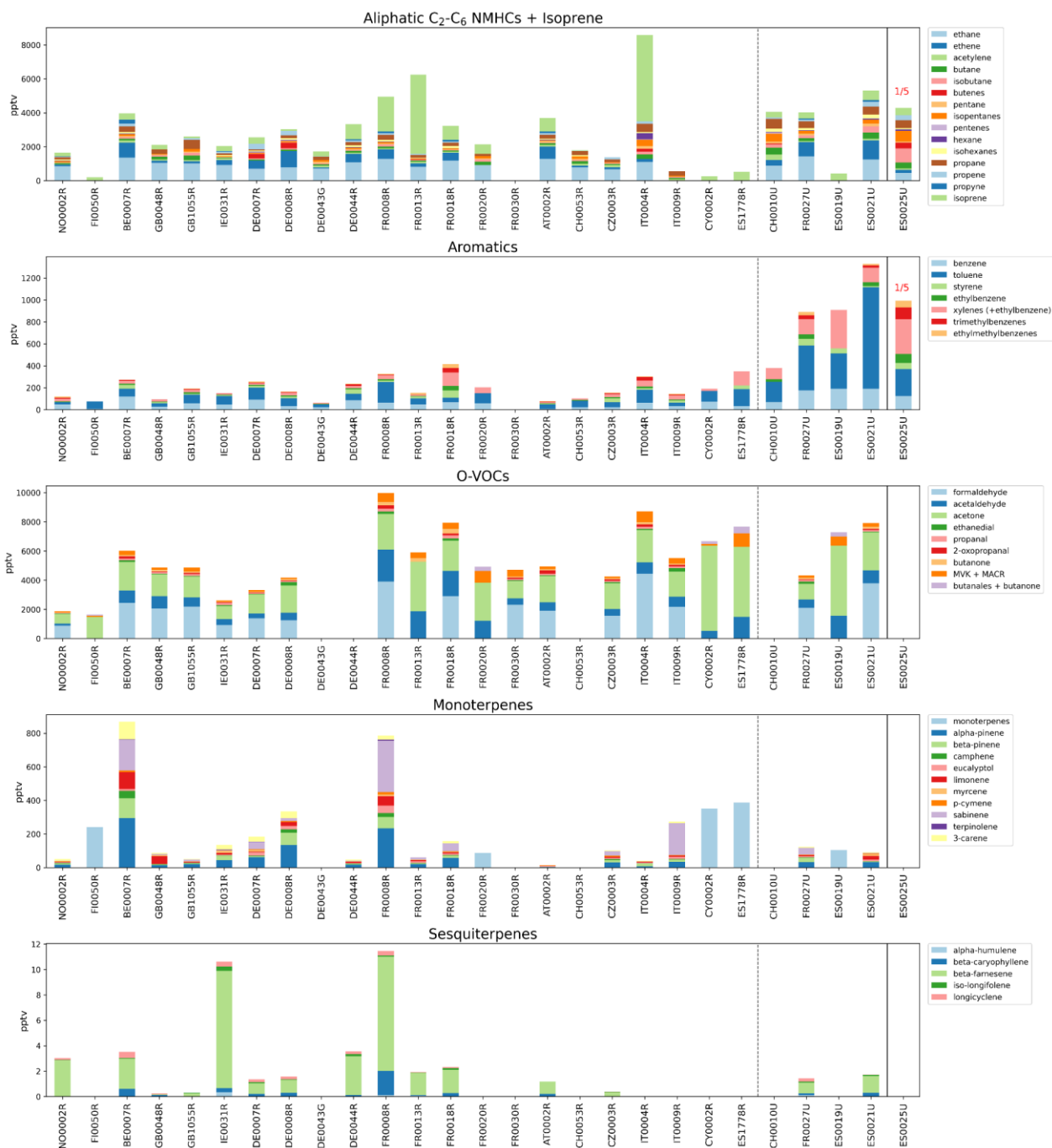
Fig. 34. Chemical composition of different VOC groups at all sites, averaged over the measurement period (12-19 July 2022). The sites are sorted from north to south, with the urban sites separated to the right. The NMHC and aromatic measurements at ES0025U were divided by five. MVK is 3-buten-2-one, MACR is 2-methylpropenal, and MEK is butanone. The different trimethylbenzenes and xylenes were summed. The xylenes for the PTR-MS sites also include ethylbenzene. Note that not all sites include all components, most notably isoprene was missing at some sites, while PTR-MS sites include isoprene only; besides, some O-VOCs sites missed formaldehyde data.
