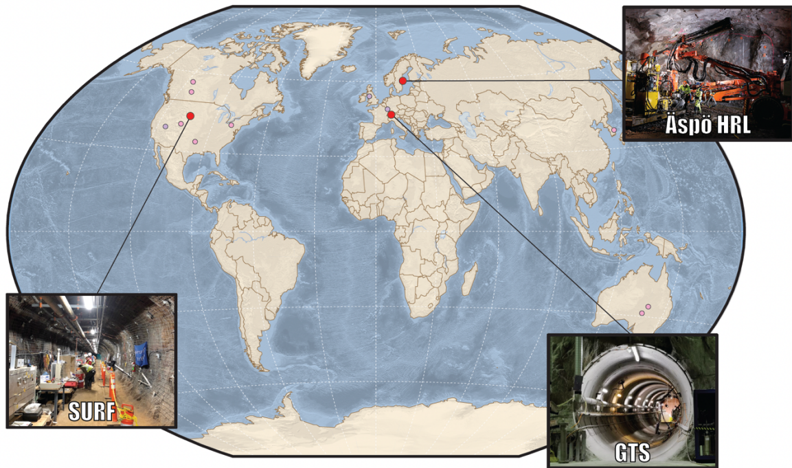
359 Figure 3. Global locations of datasets. Locations of the test sites considered: the Äspö Hard Rock 360 Laboratory (Sweden), Sanford Underground Research Facility (South Dakota, USA), and the Grimsel 361 Test Site (Switzerland). Supporting locations from past studies (Schultz, 2024; Schultz et al., 2025), 362 are also shown. 363
