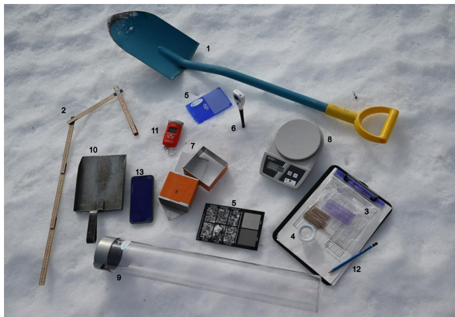
Figure 2: Measurement equipment: 1. Shovel for digging the snow pit, 2. Folding ruler for measuring snow height, 3. Toothpicks for marking layer interfaces, 4. Magnifying lens for classifying grain size and type, 5. Crystal card with 1 mm and 2 mm reference grid for classifying grain size and type, 6. Digital thermometer to measure air and snow temperature, 7. Density cutter to measure weight of a fixed volume and estimate the density, 8. Digital scale to measure the weight of the snow within the density cutter, 9. Snow water equivalent tube to take a snow sample through the whole snowpack for bulk density, 10. Flat shovel used whenever snow was higher than the length of the tube, 11. Digital scale to measure weight of snow in a plastic bag sampled with the tube, 12. Paper and pen for note taking, 13. Mobile phone to take documenting pictures. Photo credit: Lisa König.
