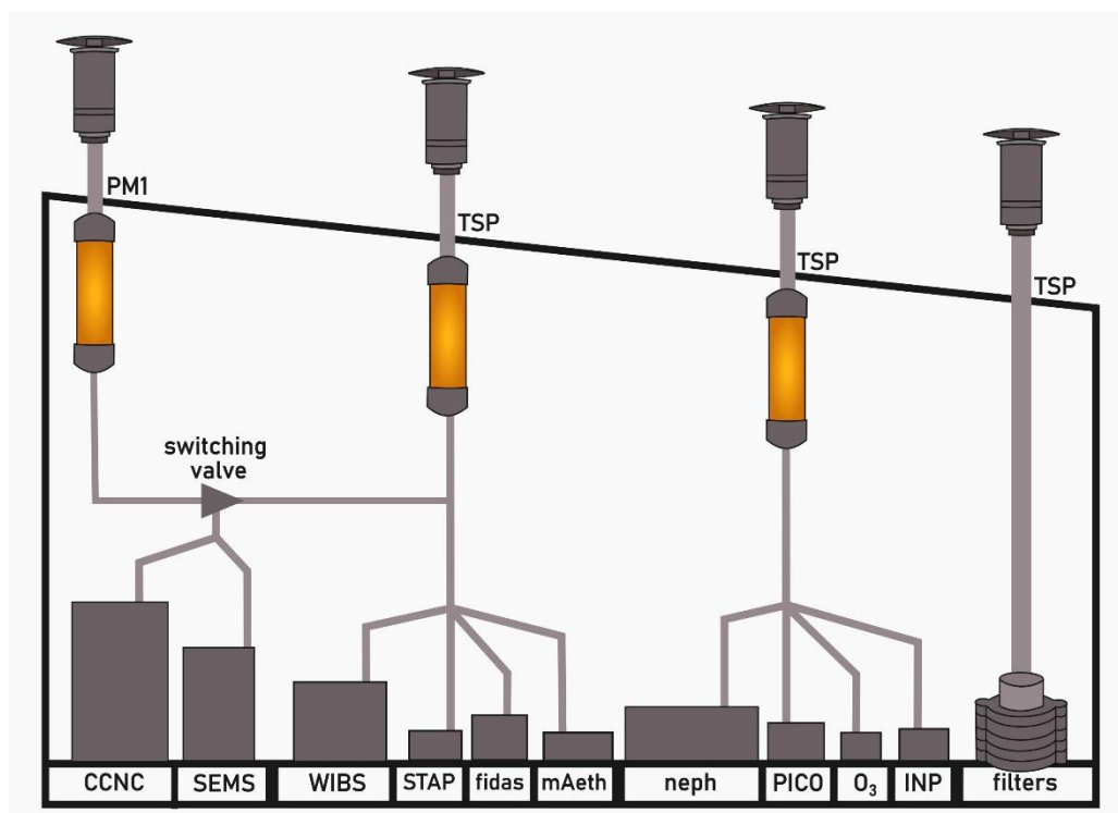
Figure S1. Schematic of the instrumental setup inside the measurement hut at NIRS. All four aerosol inlets are shown and their connections, via Silicagel dryers (orange), to the instruments. CCNC: Cloud Condensation Nuclei Counter, SEMS: Scanning Electrical Mobility Spectrometer; WIBS: Wideband Integrated Bioaerosol Sensors; STAP: Single-channel tricolor absorption photometer; fidas: Fidas Frog fine dust monitor; mAeth: micro aethalometer; neph: nephelometer; PICO: MIRA Pico Nitrous Oxide and CO gas analyser; O 3 : ozone monitor; INP: Ice Nucleating Particle filter sampler; filters: cascade impactor.
