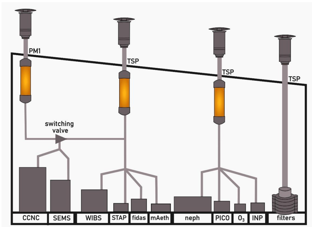
Figure 2. Schematic of the instrumental setup inside the measurement hut at NIRS. All four aerosol inlets are shown and their connections, via Silicagel dryers (orange), to the instruments. CCNC: Cloud Condensation Nuclei Counter, SEMS: Scanning Electrical Mobility Spectrometer; WIBS: Wideband Integrated Bioaerosol Sensors; STAP: Single-channel tricolor absorption photometer; fidas: Fidas Frog fine dust monitor; mAeth: micro aethalometer; neph: nephelometer; PICO: MIRA Pico Nitrous Oxide and CO gas analyser; O 3 : ozone monitor; INP: Ice Nucleating Particle filter sampler; filters: cascade impactor.
